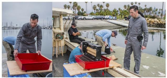
The wringer was mounted on a sturdy piece of plywood with a hole drilled and aligned beneath the drain for the wringer's collection basin. The plywood was secured on one side to the boat's gunnel with screws and on the other side to a crab crate using zip ties. Wood pieces were installed on two sides of the wringer to prevent motion starboard or portside, and clamps were attached to prevent motion toward the bow or stern. A customized funnel with a threaded spout was affixed
